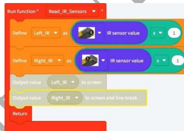
Fig. 18.44 Function “Read_IR_Sensors” used for the Avoider projects.
