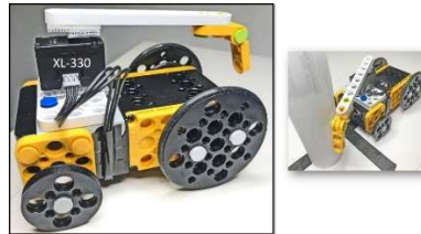
Fig. 18.67 Line-Tracker with Object Detection and Object Clearing using an XL-330.
