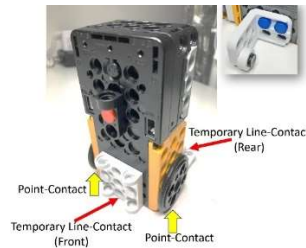
Fig. 5.6 Selected Features of “Mod-Knight” as a Motion Platform.
