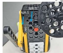
Fig. 5.4 Mod-Knight can only “see” via NIR sensor #3 and #5.
