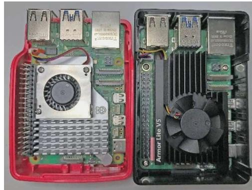
Fig. D.1 RPi and GeekPi cases for the RPi5.
