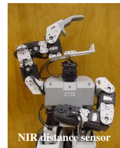
Fig. 4 – Bot “Teal’c” with Gripper (right hand) and NIR distance sensor (left hand).
