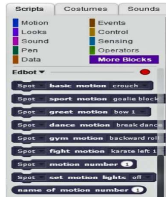
Fig. 8.8 EDBOT provides 20 Stack Blocks and 7 Reporter Blocks.
