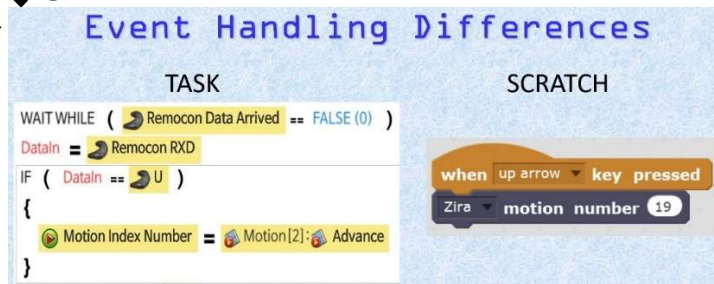
Fig. 8.16 Event Handling Differences between TASK and SCRATCH+EDBOT.
