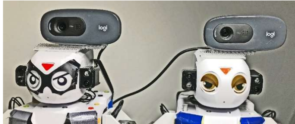
Fig. 8.89 Zira and Zork equipped with webcams mounted on their head pieces.
