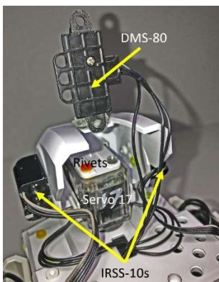
Fig. 2.5 Attaching IRSS-10 and DMS-80 Sensors to MINI Head Part.
