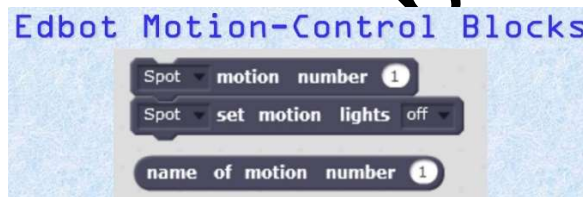
Fig. 8.11 EDBOT's Motion Control Blocks.
