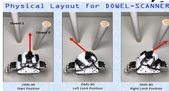
Fig. 6.84 Physical Layout and Constraints for Program “M_DowelScanner.tsk3”.
