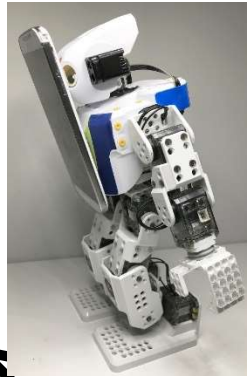
Fig. 2.6 Attaching a mobile device to the MINI robot will make it lean more forward.
