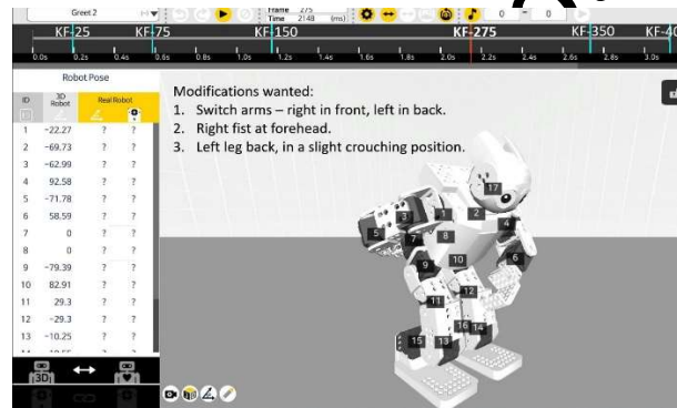
Fig. 4.30 Modifications made to Motion Unit “Greet2” to create a “Crouching Bow”.
