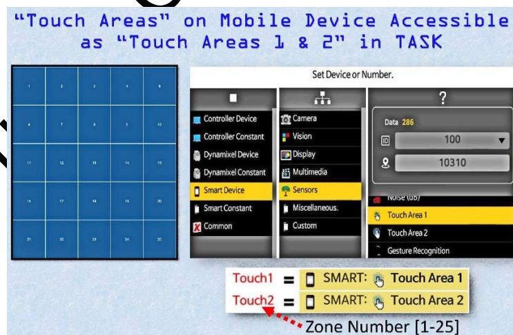
Fig. 7.12 Accessing & Programming Touch Areas on Mobile Display.
