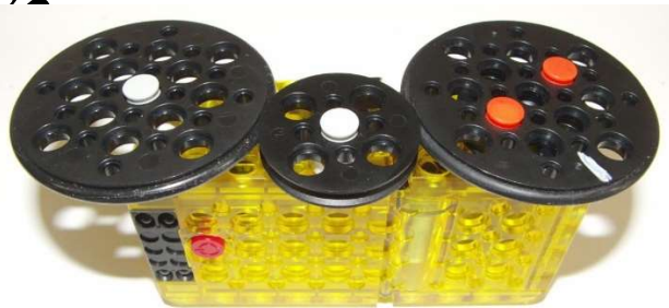
Fig. 5.7 Gear Train built from Pulley Wheels and Rubber Tires.
