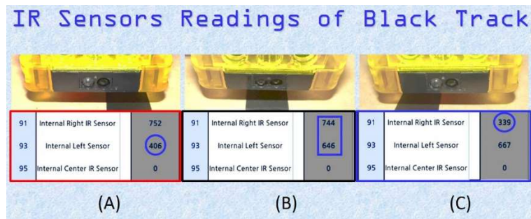
Fig. 3.56 Values for L-R-C IR Sensors for 3 configurations between CarBot and Black Track.
