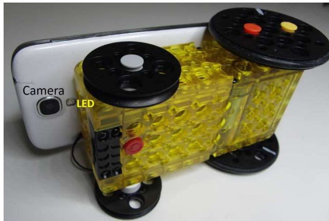
Fig. 3.60 Bottom View of a CarBot equipped with a Smartphone.
