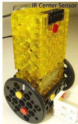
Fig. 3.9 “Spinning Top” robot and its IR Center Sensor.
