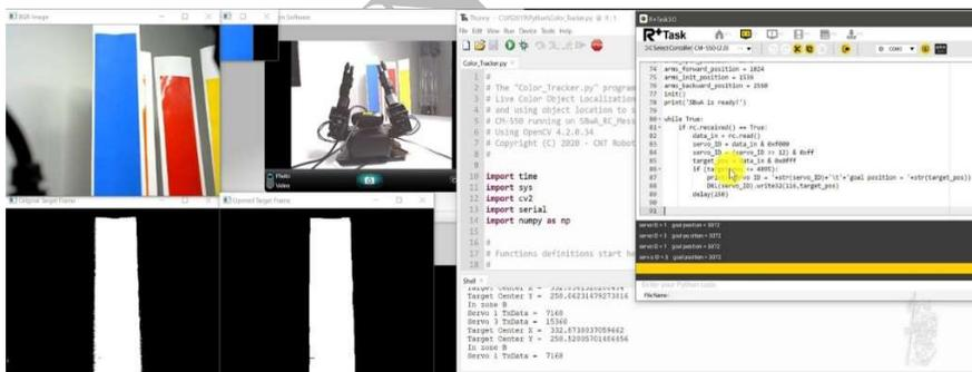
Fig. 1.8 SBwA robot running a Python/MicroPython application using OpenCV and PySerial.
