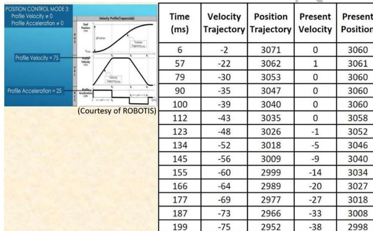
**Fig. 2.14** Typical results for “TRAPEZOIDAL” Position Control mode 3 during the first 199 ms.
