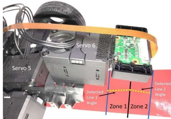
**Fig. 3.31** Pi Camera’s Setup for Color Line/Track Detection.
