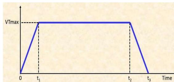
**Fig. 2.20** Velocity Trajectory definition for a Time-Based Position Control option (i.e. PC Modes 4-1, 4-2 or 4-3).
