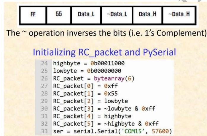
Fig. 2.66 Python's BYTEARRAY implementation of ROBOTIS Remocon Packet.
