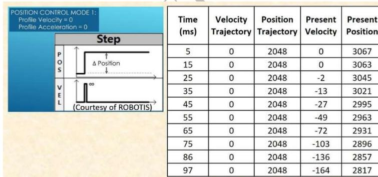
**Fig. 2.3** Typical results for “STEP” Position Control mode during the first 100 milliseconds.
