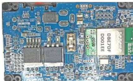
**Fig. 1.1** Bottom view of CM-550 showing the embedded BT-410 module on the right.
