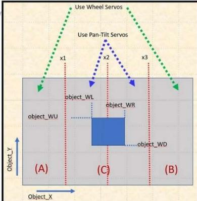
Fig. 3.78 Parameters used in the VSR Algorithm of “PTC\_RC\_VSR\_SD\_RPi\_CD.py”.
