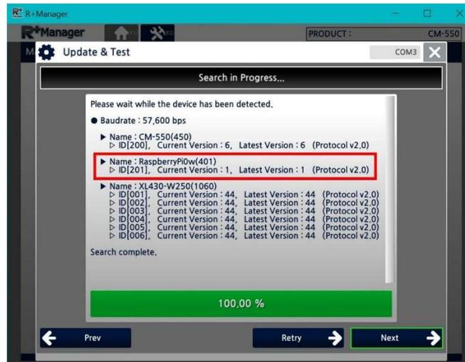
Fig. 3.2 MANAGER shows connection to the RPi Zero W as DXL(201).
